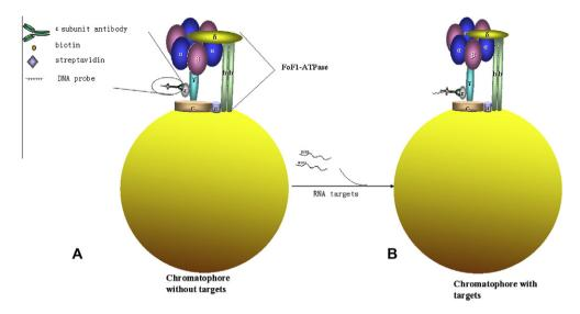
Fig. 1. Schematic illustration of the rotary biosensor. (A) Rotary biosensor without targets. (B) Rotary biosensor with targets.
